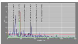
We need to emphasize at this time that frequencies at 843, 2530, 3370 cpm may be serious carrier bearing defects. The carrier bearing appears to be the weak link in the unit. We did see the 843 at an earlier inspection, but it was not present at the next inspection. Bearing defects do get better before failure.
