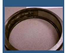
Outer race bearing defect of gear A bearing found through vibration analysis
