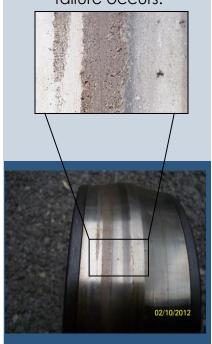
Inner race bearing defect of held bearing found through vibration analysis
